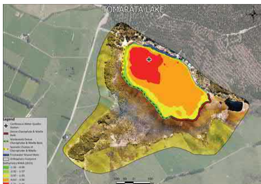
This compiled model is a combination of the lake bathymetry and wetland point cloud. It integrates various data sources and survey results into a single geospatial platform. It is used to display and analyse multidisciplinary data and is the backbone of the project.
