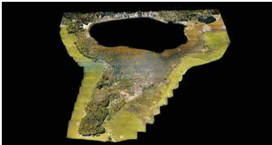
Drone imagery was used to create a 3D point cloud model of the lake and wetland. This high-resolution imagery creates a geospatial representation of the entire ecosystem.
