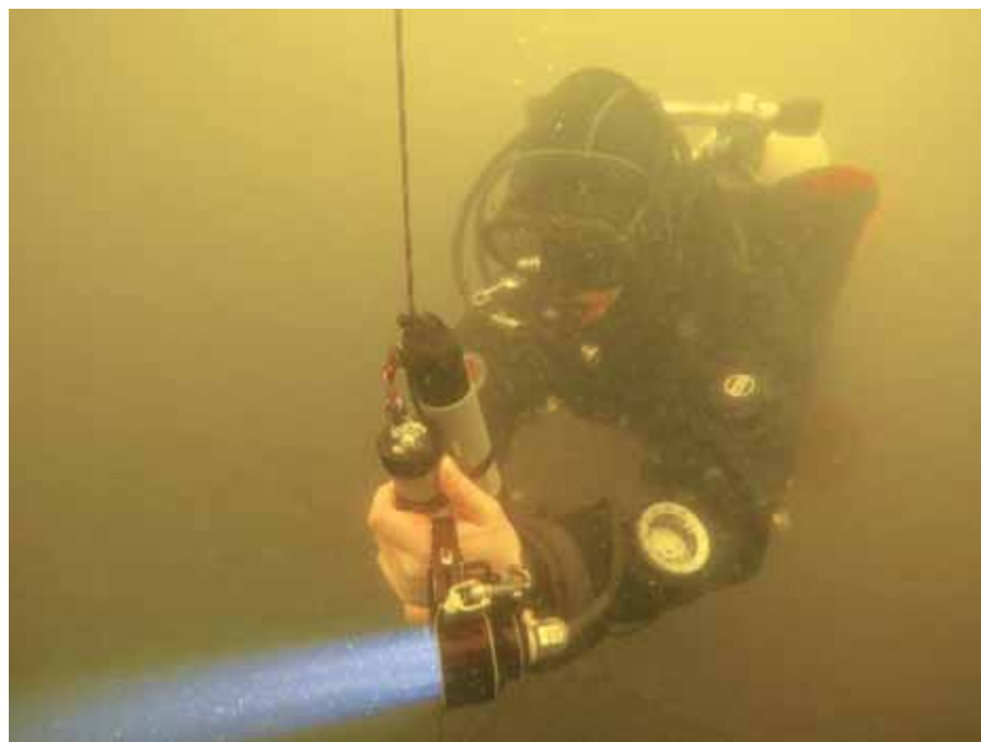
Louise Greenshields installs water quality sensors that monitor pH, temperature, dissolved oxygen and light every 15 minutes. This data will be used to create an in-lake process-based model.
